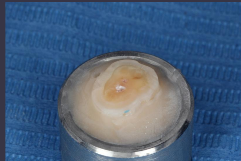
Cohesive breakage of composite rode in group 1 sample (delayed)
